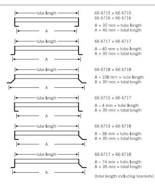
The tube length and bracket centres (A) have an important bearing on manufacturing, installation and ordering. The bracket spacing (A) is measured from the centre of the screw hole of one bracket to the centre of the screw hole of the other bracket. The tube length is calculated from the bracket centres (A) by adding or subtracting the differential dimensions provided here.
